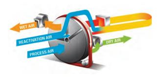
The DS system uses two independent air flows. The main air flow will be dried, the secondary air flow of lesser volume will be used to evacuate the moisture retained by the desiccant rotor.
